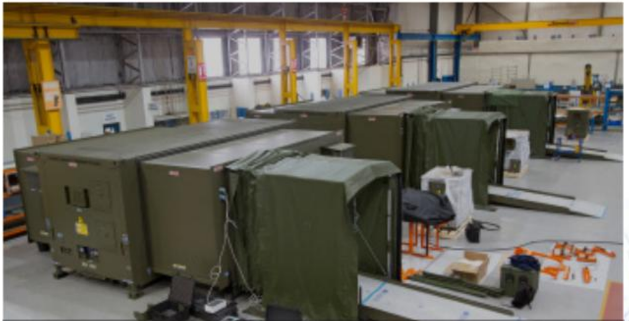
3 French CT Scanners prior to delivery to the customer. Marshall was awarded a Queen's Award for Innovation for the design which enables the scanner to be up and running within four hours of arrival. The company has worked closely with Phillips Healthcare developing this life saving capability to the UK and Norway with other customers in the pipeline.
