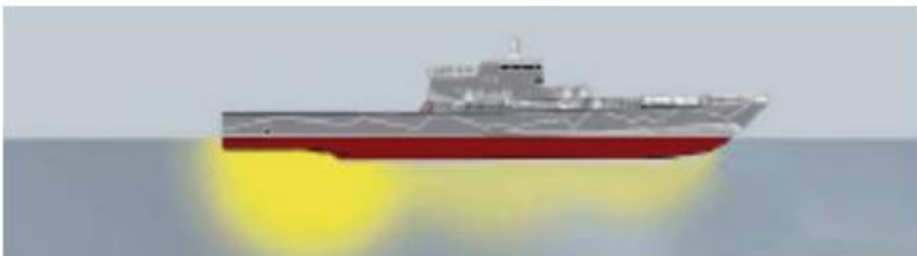
Illustration of an UEP signature of a vessel
